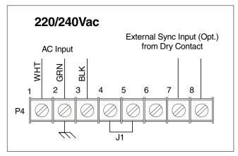
Figure C-2 Wiring the 24A715/M for 220/240Vac Operation
